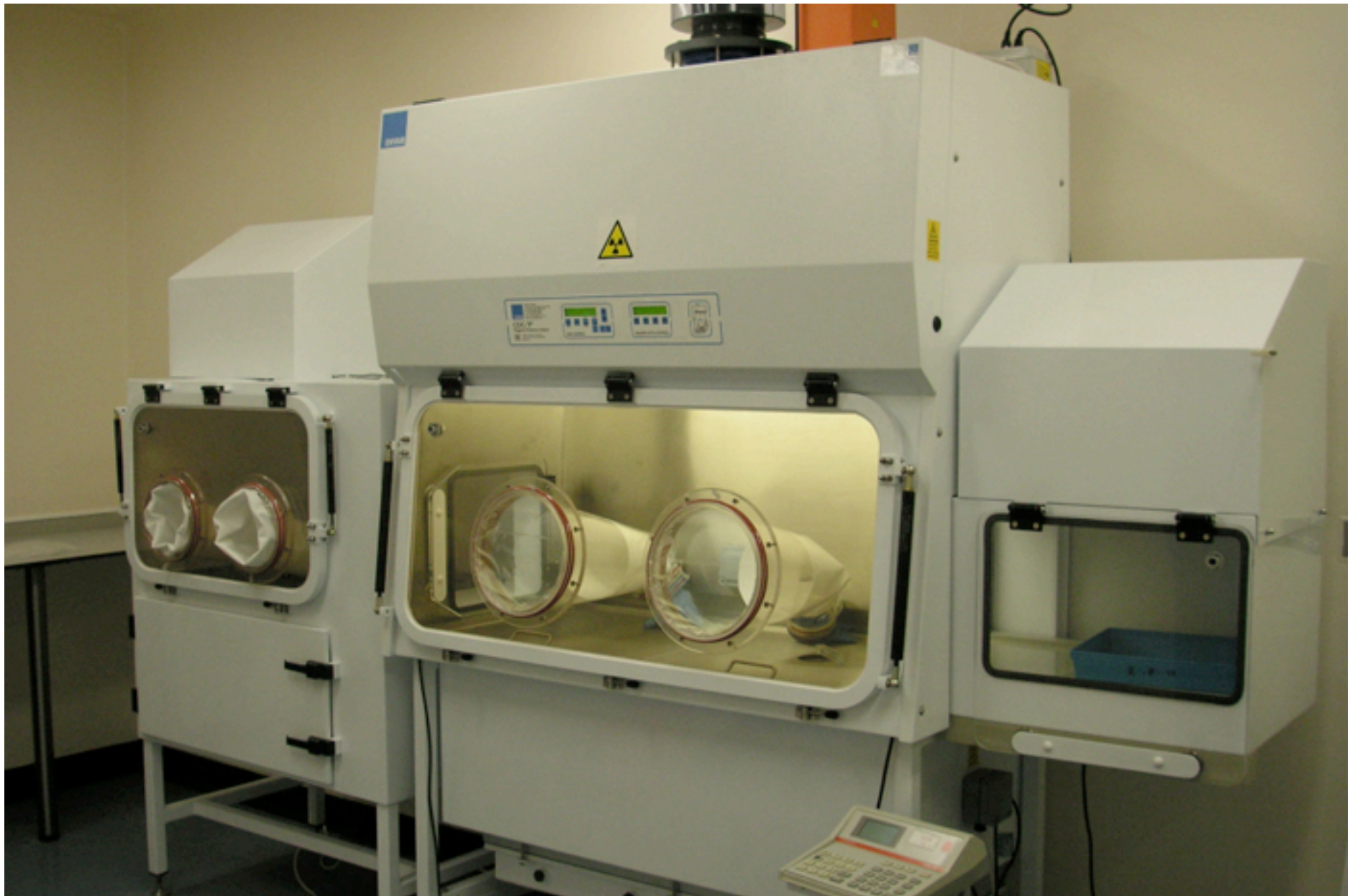
2 –glove Technetium isolator
